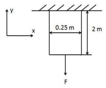
The plate is so thin that there is no significant stress variation through the thickness. Gravity effects are significant.
