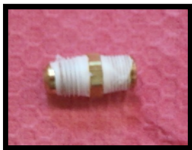
Figure 6: Teflon Tape on Connector
