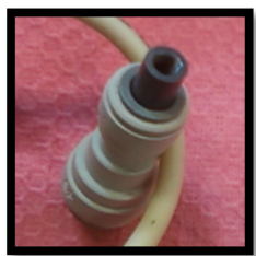
Figure 7: Carburetor Connector Manufactured from PVC
