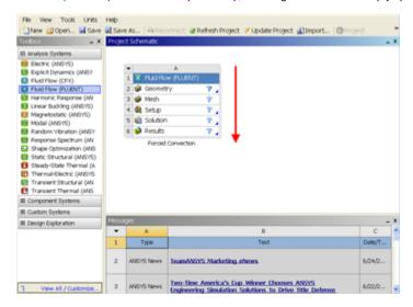
Since we selected Fluid Flow (FLUENT), each cell of the system corresponds to a step in the process of performing CFD analysis using FLUENT. Rename the project to Forced Convection.
