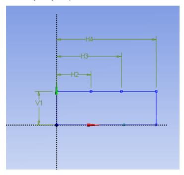
Under Details View in the lower left corner, input the values for the appropriate dimensions. Then hit enter each time each dimension is entered.
