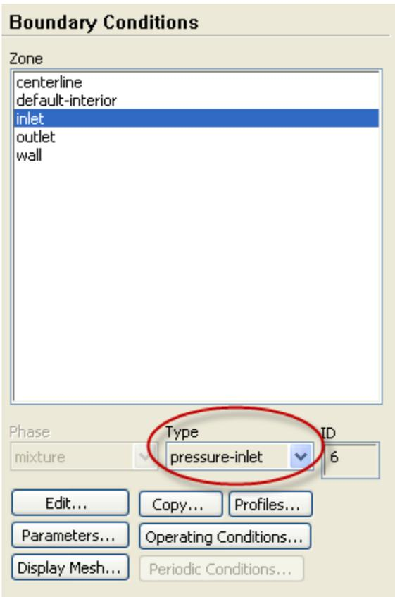
Select *inlet* under **Zone** and pick *pressure-inlet* under **Type** as its boundary condition. Automatically, the *Pressure Inlet* window should come up.
