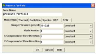
Click *OK*. The *pressure-far-field* boundary type effectively imposes that there is no upstream propagation of disturbances if the flow at the boundary is supersonic. See section 7.9 of the FLUENT help for more details about this boundary type.
