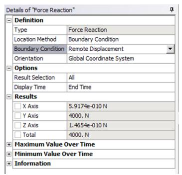
Do the same step for Remote Displacement 2 (point B).
