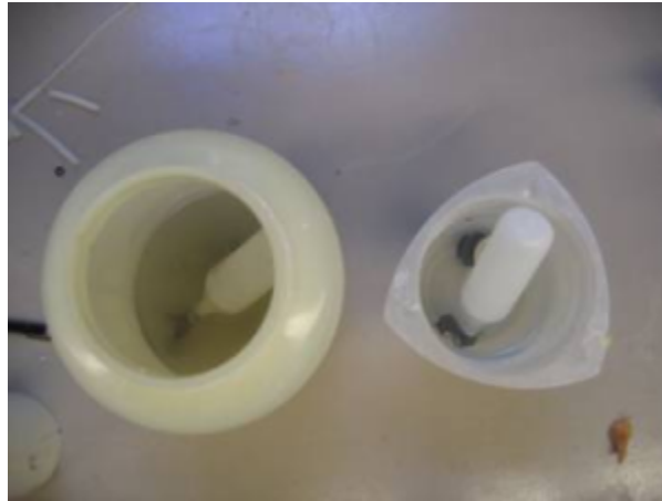
FCM- Top-down view of the float valves in chlorine (left) and alum solutions (right) for the corrosion testing (Fall 2007).
