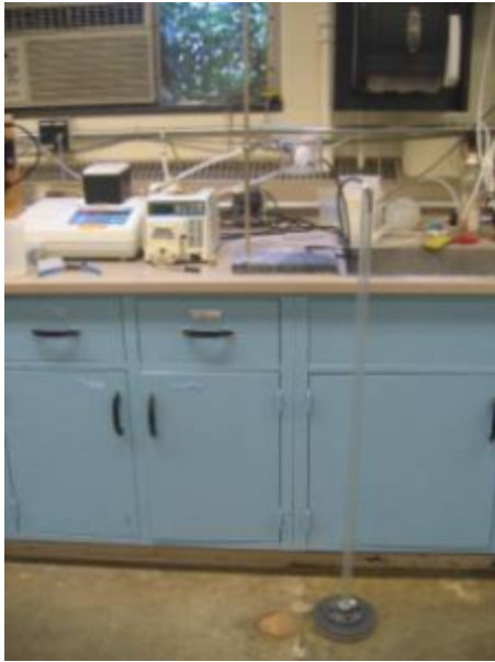
FCM- The column experimental set up for determining the relationship between flow rate and headloss (Fall 2007).
