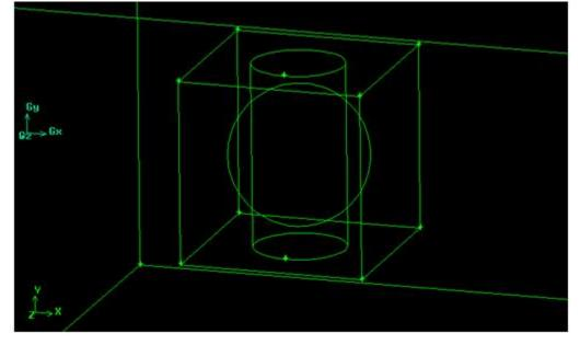
The cylinder will serve as the tool for another volume split, allowing us to separately isolate the upper and lower y-axis 'poles' of the sphere.
