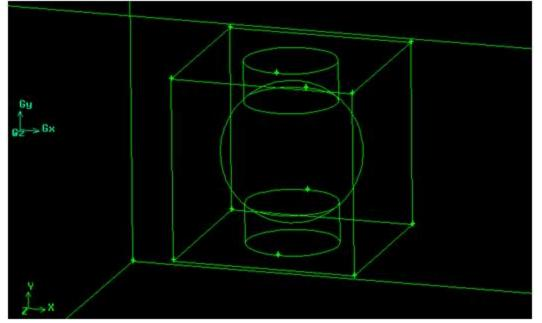
Our ultimate goal is to ensure that none of the volumes composing the sphere contain a radius = 3, circular element of the sphere. Next we need to construct a new face to further divide *sphere\_box*.
