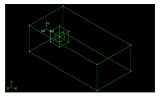
Now we want to isolate the volume contained by sphere\_box from the rest of the flow domain's volume. We can achieve this by performing a volume split.
