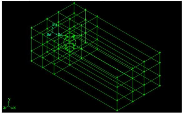
This should divide the flow domain into twenty-six, empty rectangular segments plus the box containing the sphere.
