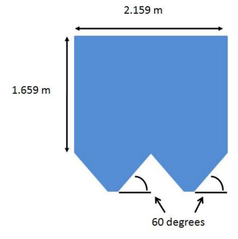
The above picture consists of relevant dimensions for AguaClara sedimentation tanks. The length into the page of the tank varies depending on the community.
