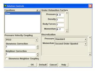
Select PISO from the Pressure-Velocity Coupling drop-down list.
