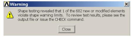
Elements that exceed shape warning limits can lead to degraded accuracy. Here it is a minor concern since only 1 element out of 682 is causing the warning. So it is reasonable to press on. In general, it is always a good idea to pay close attention to the warnings and understand their effect on your solution. As a veteran in these things, I can attest that ignoring warnings can come back to bite you in incovenient parts of the anatomy. Close the warning window.
