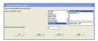
The Element Types window should list two types of elements: MESH200 and SOLID45.
