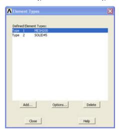
In order to set the 3-D quadrilateral with 4 nodes option for MESH200, click on MESH200 and then Options ... in the above menu. Then, select QUAD 4-NODE next to Element shape and # of nodes K1. Click OK.
