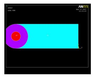
To correct any mistakes, you must click **Main Menu > Preprocessor > Modeling > Delete > Areas Only** and then pick each area you want to remove. The mouse pointer will show an up arrow for picking areas and a down arrow for un-picking areas. Right-click to switch between pick and unpick mode. When you have made all your selections, click **OK**. Click **Utility Menu > Plot > Replot** to refresh the view.
