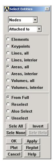
Check that only nodes attached to the front face are currently selected by clicking Replot in the Select Entities menu (this replots nodes).
