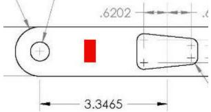
In the coordinate system in our model, let's say this area is given by -1.77" x -1.57" and 0.45" y 0.85". To find the average strain in this area, we will select all nodes that lie in this area and then list the strain values at these nodes. You can copy these values over to Excel or MATLAB to find the average value.
