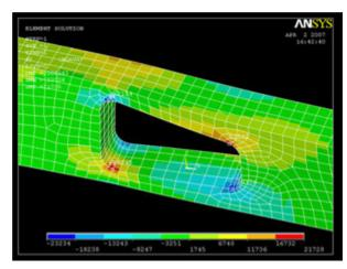
Compare the stress values with the von Mises stress. (Click on von Mises stress, then  $\ensuremath{\textit{OK}}$ )
