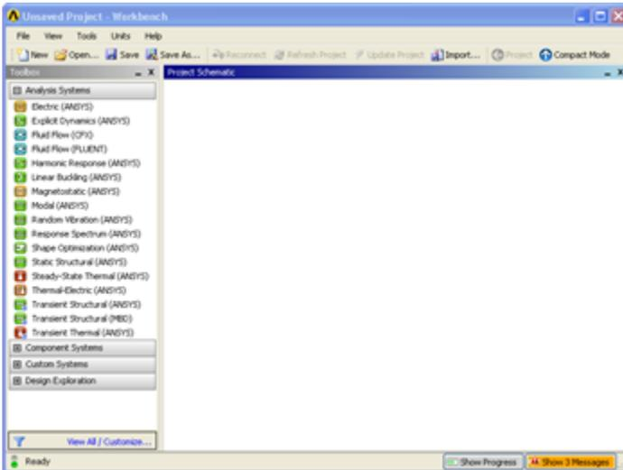
To begin, we need to tell ANSYS what kind of simulation we are doing. If you look to the left of the start up window, you will see the Toolbox Window. Take a look through the different selections. The bicycle crank is a static structural simulation. Load the **Static Structural** tool box by dragging and dropping it into the Project Schematic.
