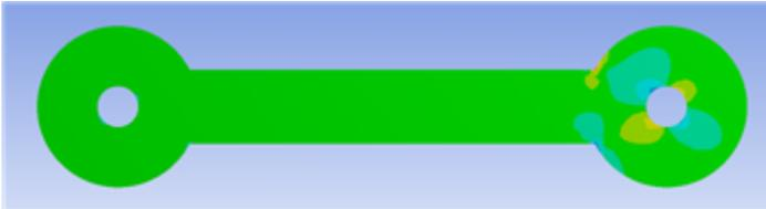
Here, we assumed that the stress was zero. If we use the probe tool to examine the middle section of the bar, we find that most of the stresses are on the order of  $1 \times 10^{-3}$ , meaning once again the simulation agrees with our calculations.
