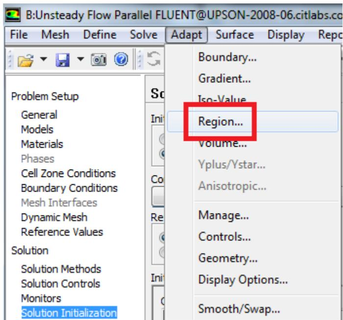
Then set **X Min** to 0.5 m, set **X Max** to 32 m, set **Y Min** to 0 m, and set **Y Max** to 32m. (Note: If you instead "patch" the region  $0.5 < x < 32$  and  $-5 < y < 5$ , the periodic vortex shedding starts much quicker; so we recommend that).
