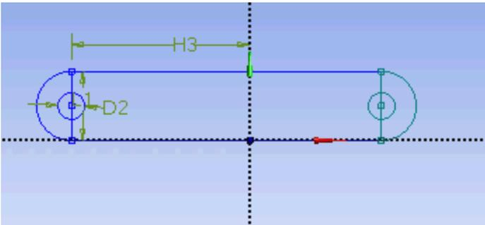
Next, we will make sure that the both circular hole is of same dimension. Under **Constraints** tab, select **Equal Radius**. Execute constraint in the **Graphics** window as shown below.
