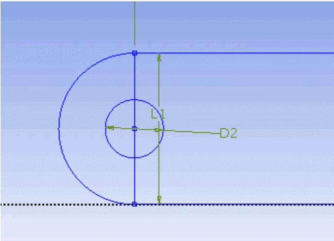
At this point, we have the outline of the crank done. We need to add the cut out in the middle of the crank. First start with a sketching of the cut-out. Under **Draw** tab, click on **Line** and execute drawing in Graphic window as shown below.
