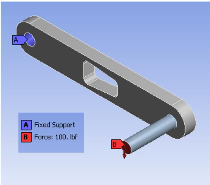
Calculate the deflection, strain and stress distributions in the crank/pedal shaft combination for this loading condition. Use the ANSYS results to evaluate the degree of stress concentration in the vicinity of the cut-out in the crank geometry.
