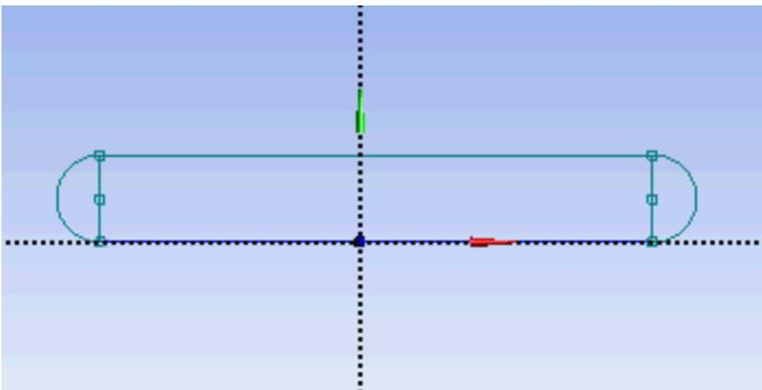
Next, we will dimension the current drawing. Under *Sketching Toolboxes*, select *Dimensions* tab. You will see a list of dimensioning options. We will use the default *General* option. Execute the geometry dimensioning as shown below.
