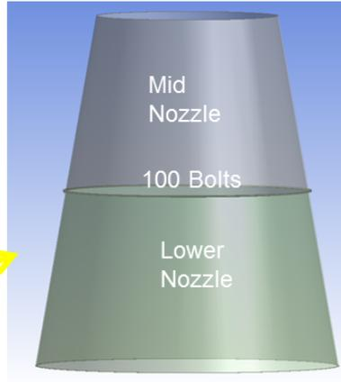
Below is close-up view of the bolted flange joint connecting the mid and lower parts of the nozzle.
