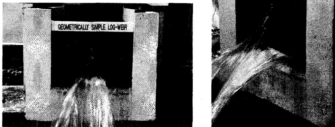
FIG. 9. Discharging Weirs: (a) Front; (b) Side
