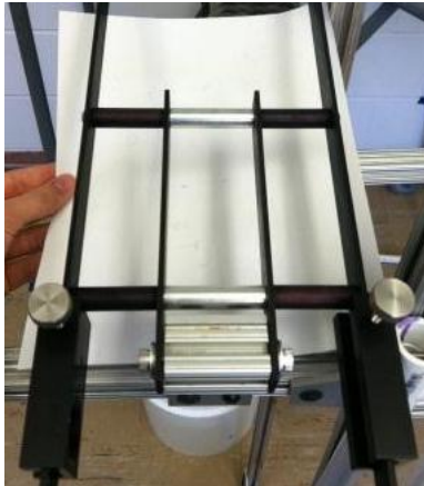
Figure 11: Lever Arm Assembly Cross Bracing
