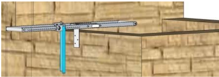
Figure 2: Lever Arm Plant Attachment
