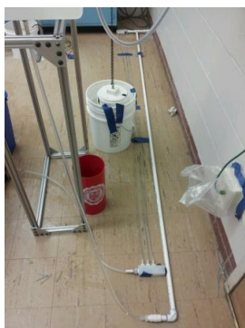
Figure 8: Large diameter tubing leading from the constant head tank to the small diameter long straight dosing tubes (3 clear PVC tubes)
