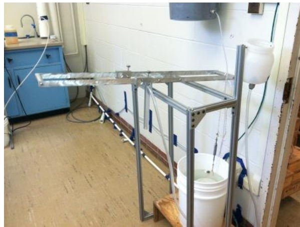
Figure 13: LCDC System Setup Pre-Anodization of the Lever Arm Assembly, with an Undersized Constant Head Tank
