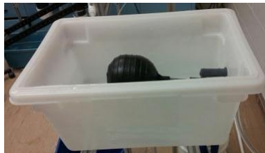
Figure 7: Constant head tank with float valve
