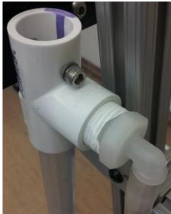
Figure 12: Rigid drop tube connection to the slider on the lever arm
