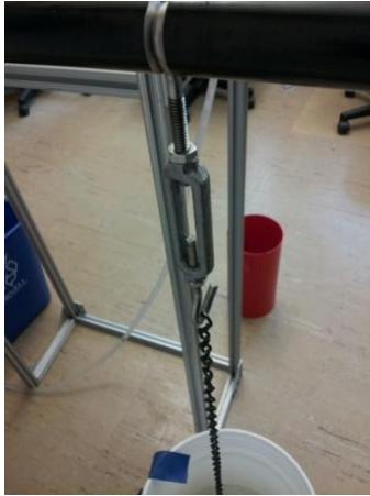
Figure 10: Turnbuckle attached to the lever arm
