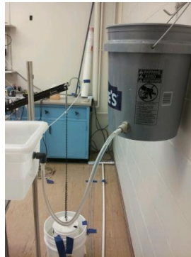
Figure 6: Chemical stock tank (gray bucket) connected to the constant head tank (white container)
