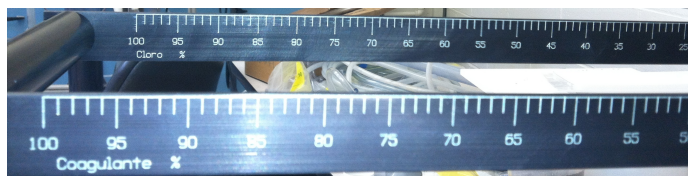
Figure 14: Anodized Lever Arm with Scale Engraving
