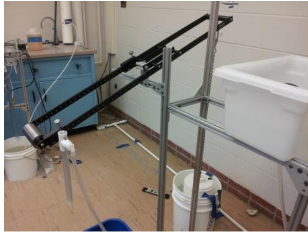
Figure 5: Maximum flow through the plant and maximum chemical dose flow through the LCDC system. Note: the slider is set at 100% dose and the level in the entrance tank is at the maximum height of 20 centimeters from the zero level
