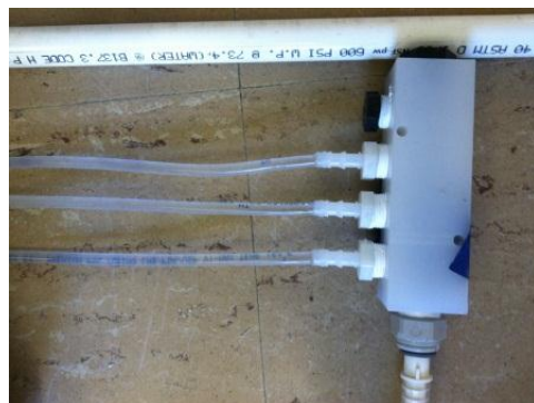
Figure 3: Manifold Smaller Diameter Tube Connection
