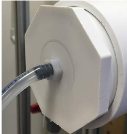
Figure 10: The barbed fitting connection originally screwed into the PVC plug.
