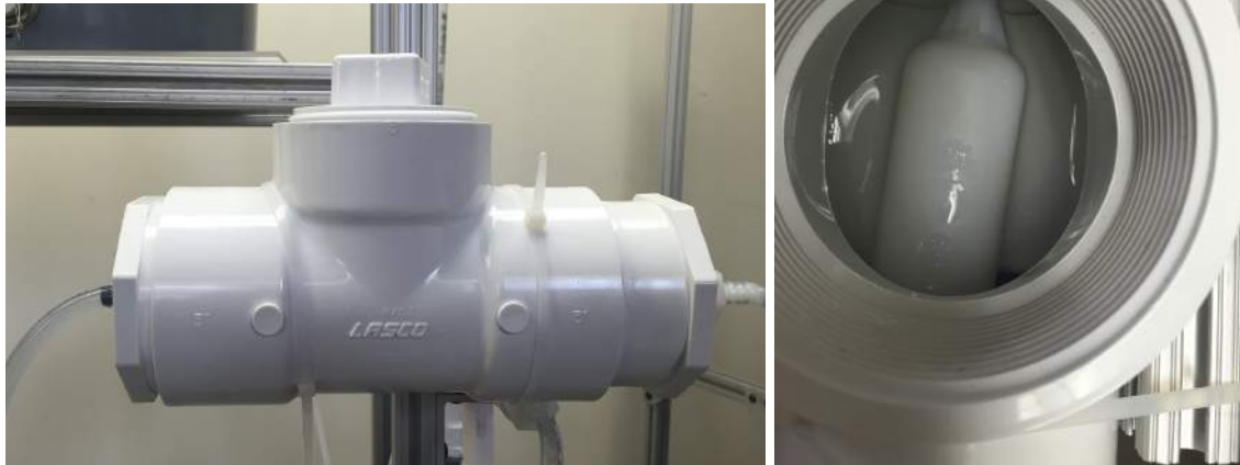
Figures 8a, 8b: From left to right: (a) the new CHT design housed by a 3" PVC tee, (b) aerial view of the mini-float valve inside of the CHT.
