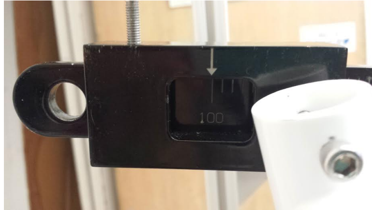
Figure 3: The slider on the lever arm should always be set to the position 100 cm to ensure accuracy of results.
