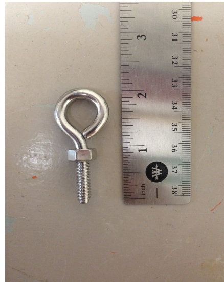
Figure 8: Type 316 stainless steel eye-bolt before experimentation.
