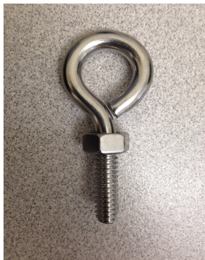
Figure 9: Eye-bolt after one week submerged in water.
