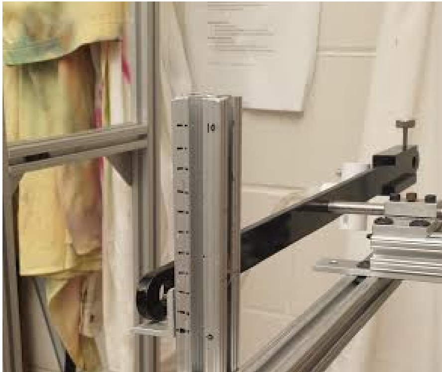
Figure 2: The stop that stabilizes the lever arm so that it is exactly parallel with the ground. This acts as a reference point for further experiments and ensures consistency.
