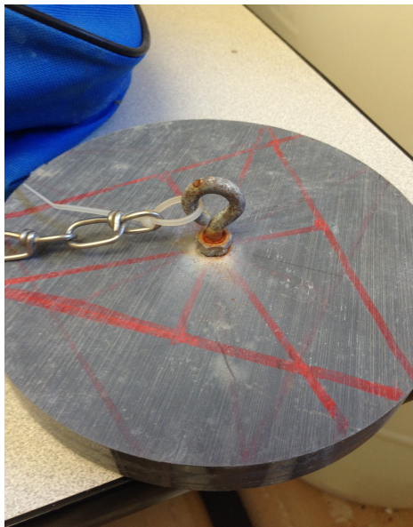
Figure 7: Rusted eye-bolt from Spring 2014 semester.
