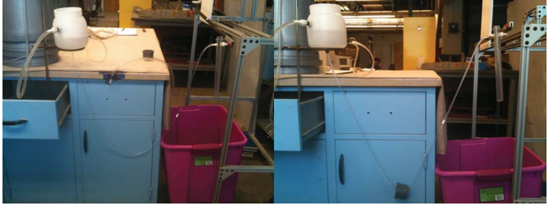
Figure 6: Fall 2011 preliminary lab setup. The single, small diameter tube is attached to the CHT by a push-to-connect at the base instead of a barbed fitting on the side. This dosing tube is then connected directly to the dose tube using a previously tested barbed fitting. The picture on the right shows the addition of a weight to reduce curvature to a single point.
