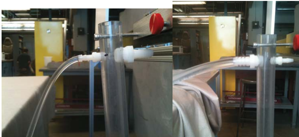
Figure 5: Two fittings that will be used in following experimental setups. The picture on the left is the drop tube with the previously tested barbed fitting. The picture on the right is the new, larger, 1/2” barbed fitting for the larger ID tube that will be connected to the smaller ID tubing.
