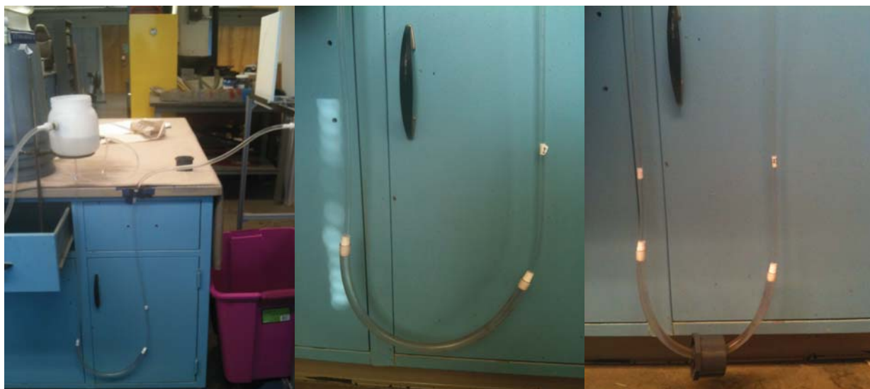
Figure 8: Fall 2011 preliminary lab setup. The single, small diameter tube is split into two, uneven sections. One longer section is attached to the CHT by a push-to-connect at the base instead of a barbed fitting on the side. This dosing tube is then connected to a \frac{1}{2} in ID tube by using a small section of \frac{3}{8} in ID rigid tubing, which is then curved to complete the 180-degree turn. The shorter segment of small diameter tube is connected to this and then connected to the \frac{1}{2} in dosing tube. The picture to the far right shows how the addition of a weight reduces curvature in both tube segments.
