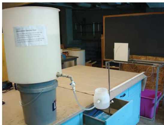
Figure 1: Summer 2011 experimental apparatus. Small diameter tube(s) between the CHT and drop tube are straight in the white trough. This setup will be continued to be used for the preliminary experiments to test the validity of the viscosity tests and data evaluated by the Summer 2011 team.
