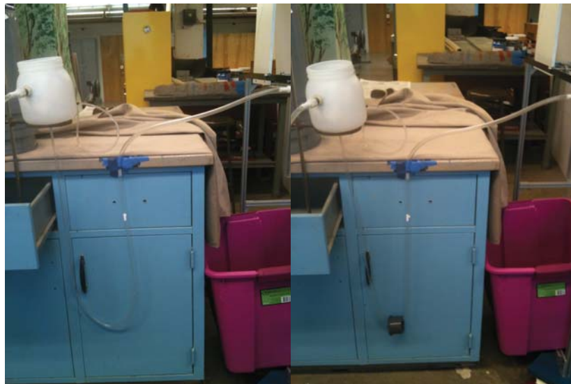
Figure 7: Fall 2011 preliminary lab setup. The single, small diameter tube is attached to the CHT by a push-to-connect at the base instead of a barbed fitting on the side. This dosing tube is then connected to a \frac{1}{2} in ID tube by using a small section of \frac{3}{8} in ID rigid tubing. The picture on the right shows the addition of a weight to reduce curvature to a single point.
