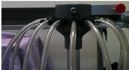
Figure 3: Detailed image of reducer with nine small diameter tubes connected
