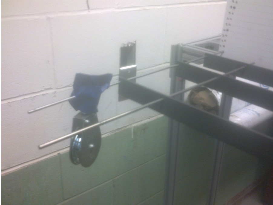
Figure 2: 500 gm pulley used as weight used to ensure uniform horizontal level across lever arms
