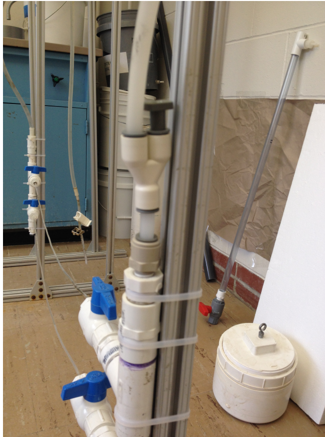
Figure 4: Y-channel Air Removal System
