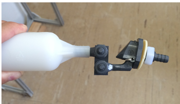
Figure 1: PVC Screws and Bolts on Float Valve
