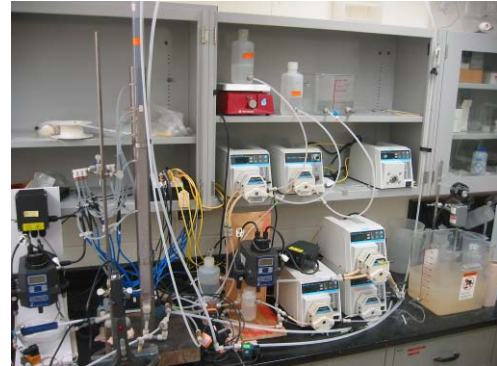
Figure 8. Sand filtration unit with backwash pretreatment and direct filtration capabilities.
