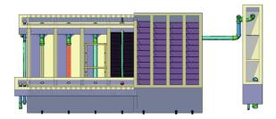
The AguaClara technology included in each design consists of gravity powered dosing of coagulant, hydraulic rapid mix (to blend the coagulant with the contaminated water), hydraulic flocculation (to form large aggregates
