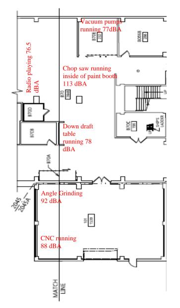
Results with no equipment running were between 70-72 dBA. Room B70 experienced levels between 95-97 dBA with the chop saw running inside of the paint booth.
