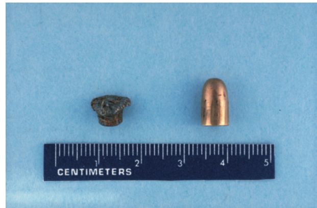
FIG. 7-30 Illustration of bullet performance on impact with bone. The bullet on the left is an unjacketed .22 handgun bullet that traversed the abdomen of a cat before striking the wing of the ilium. The bullet on the right is a .25 caliber fully jacketed bullet that fractured a lumbar vertebra. Note the lack of deformation compared with the soft-lead .22 slug. (Source: Pavletic 1986.)
