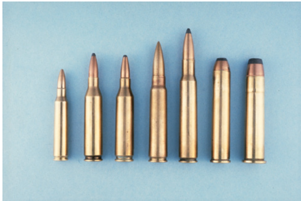
FIG. 7-31 Various rifle rounds (from left to right): 5.56 mm full-patch M-16; .243 Winchester hunting; 6.0 mm hunting; .30 military, armor piercing; .30-06 Springfield hunting; .44 Marlin hunting; .45-70 Government hunting. The partial copper jacket of the sport or hunting bullet provides controlled expansion of the exposed lead core on impact. (Source: Pavletic 1986.)
