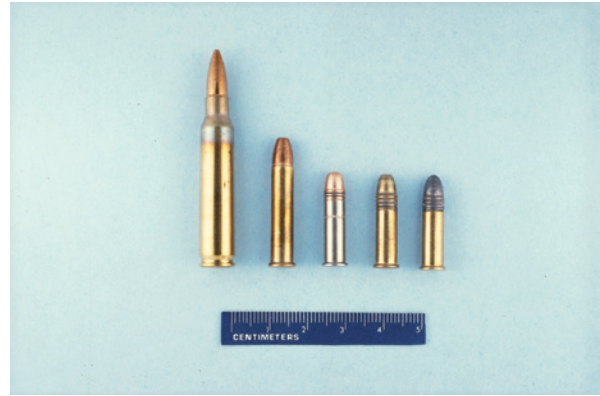
FIG. 7-33 These .22 cartridges demonstrate the various sizes and designs of these rounds (left to right): 5.56 mm (.223), 55 grain, full-patch centerfire M-16; .22 Magnum jacketed rimfire; .22 Winchester long rifle high power, 29 grain hollow point; .22 Remington long rifle, high velocity, 36 grain hollow point; .22 long rifle with uncoated lead bullet. The .22 Winchester and .22 Remington have a metallic coating that has little influence on minimizing bullet deformation. The decorative coating is reported to shun dirt, grit, and lint. A waxy coating or priming on the rimfire long rifle illustrated lubricates the bullet and minimizes fouling of the gun barrel. Note that the .22 designation does not indicate the projectile's weight, composition, design, or velocity, only its diameter. (Source: Pavletic 1986.)
