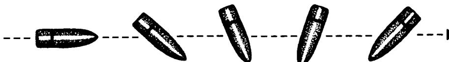
FIG. 7-43 Schematic diagram illustrating tumbling (forward rotation around the center of the mass). This unstable flight pattern increases the projectile's surface presentation to the target, enhancing tissue damage. (Source: Swan KG, Swan RC. 1980. Gunshot Wounds . Littleton, MA, PSG Publishing. Modified with permission).
