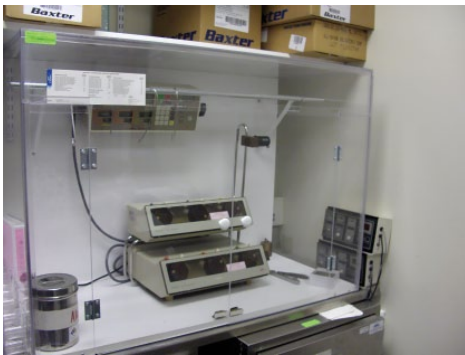
Figure 11.1 An automated parenteral nutrition compounding machine can facilitate accurate and safe compounding of admixtures.
