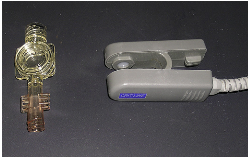
Fig. 8. A Crit-Line blood chamber ( left ) and the Crit-Line sensor ( right ) that is attached to the blood chamber to detect hemoglobin and oxygen saturation.
