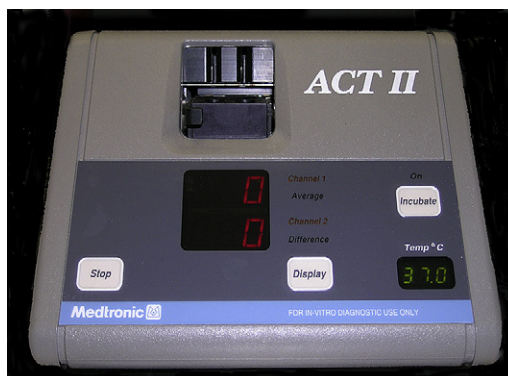
Fig. 9. ACT II monitor to measure activated clotting time.
