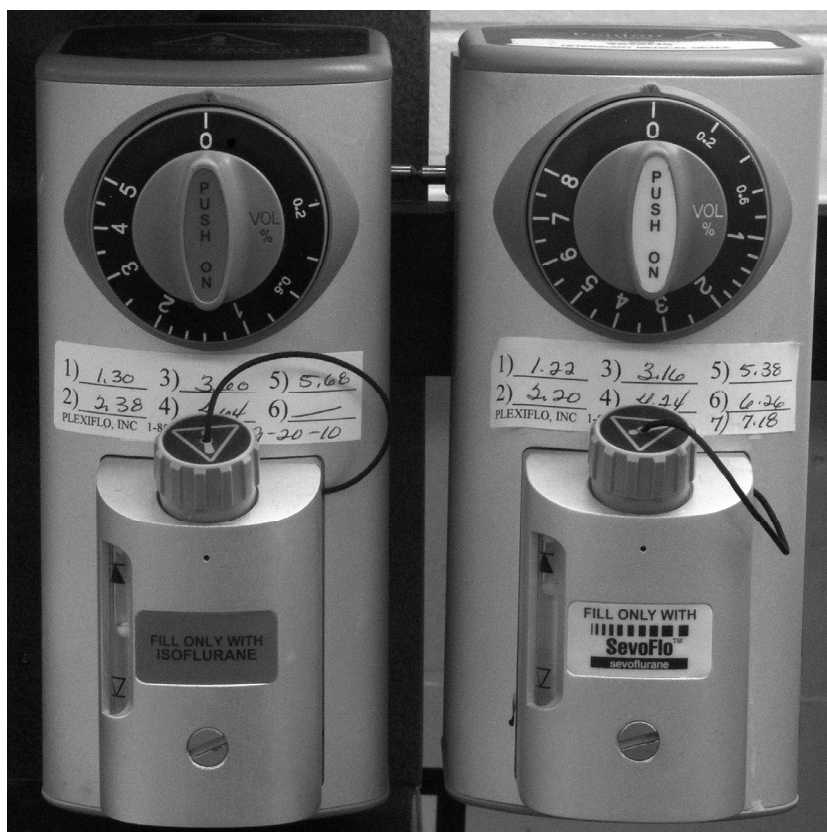
Figure 10.12 Precision vaporizers for isoflurane and sevoflurane. The dials indicate % output of each vaporizer. The handwritten labels below the dials note the actual % delivered at each setting at the time of the last scheduled machine check.
