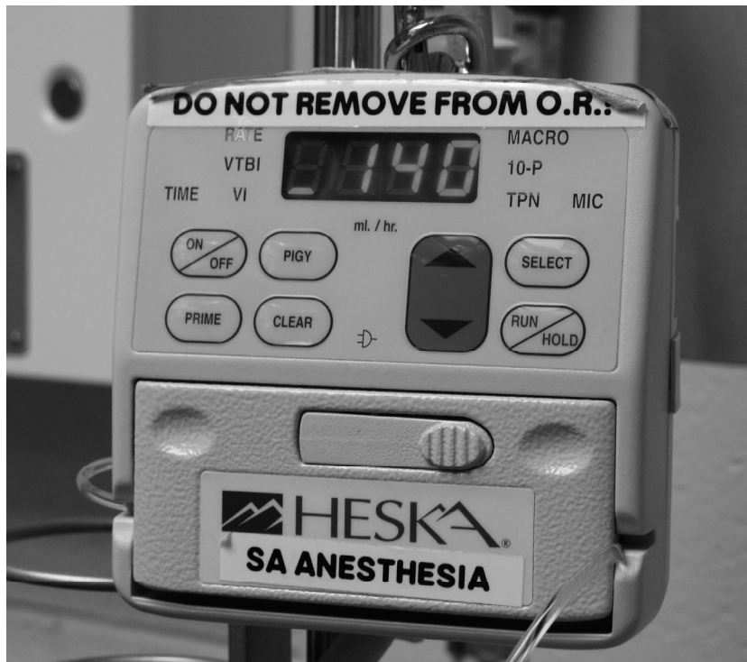
Figure 10.5 Volumetric or constant infusion pump. Devices may warn of the presence of air or occlusion of the infusion line.
