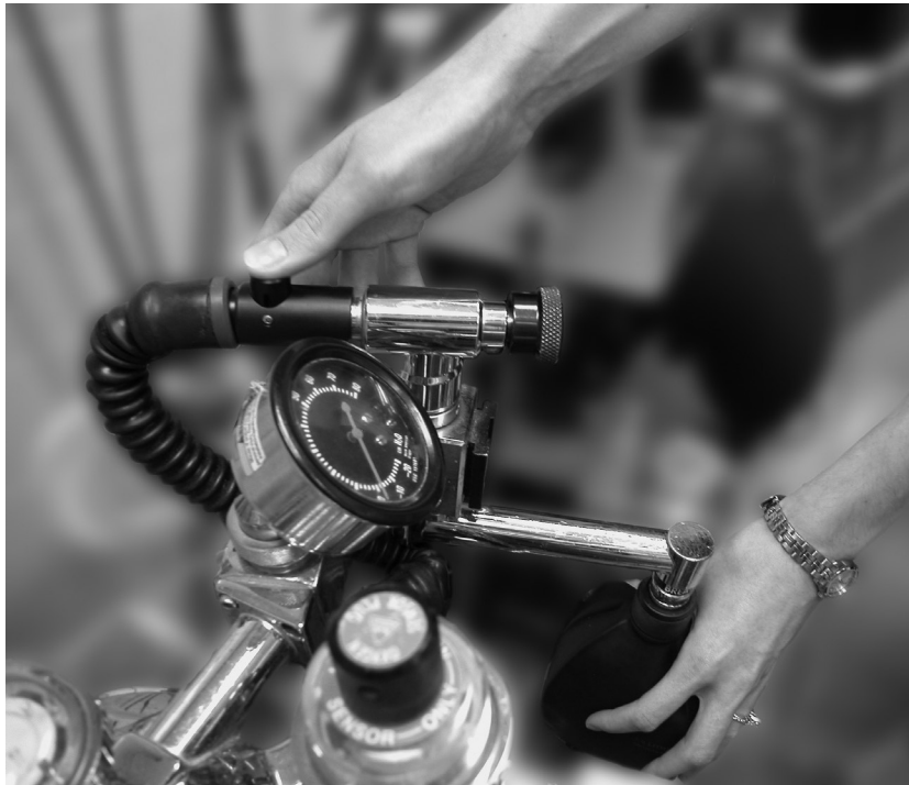
Figure 10.14 The anaesthetist is depressing the 'quick-close' button of the pop-off valve with the thumb of one hand while squeezing the reservoir bag to inflate the dog's lungs with the other hand.
