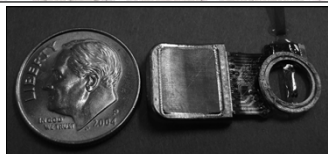
An implantable retinal prosthesis assembly showing the titanium case, external flexible circuit, RF coils and electrode array
