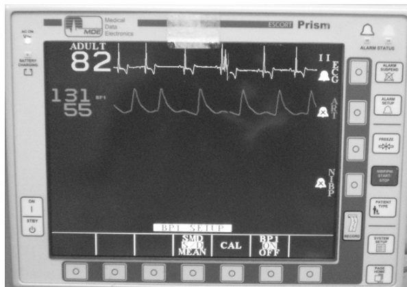
Figure 9.2 Hemodynamic monitor screen capture demonstrating standard output of arterial waveform with systolic and diastolic pressures displayed.
