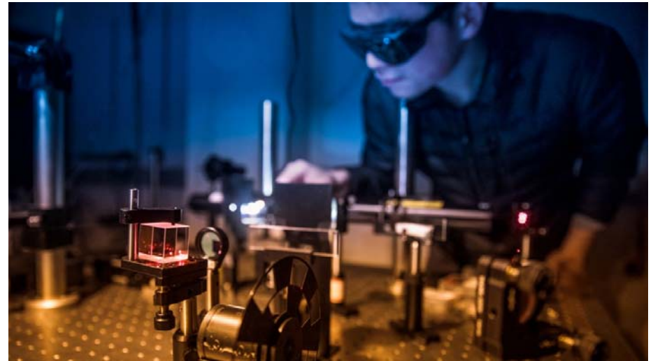
Shengwei Jiang, postdoctoral researcher, aligns an optical setup for magneto-optical Kerr rotation microscopy measurements on atomically thin magnets
