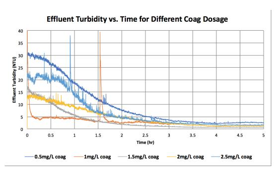
Figure 11: Effluent turbidity change vs time for different coagulant dosages ranging from 0.5 mg/L to 2.5 mg/L at 5 mg/L HA
