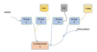
Figure 3: Schematic of experimental apparatus. The second turbidimeter is not shown.
