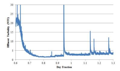
Figure 10: Effluent turbidity as a function of time with 5 mg/L of humic acid and 2.5 mg/L of coagulant. This set of experiment yielded a lowest effluent turbidity value of 1.36 NTU.
