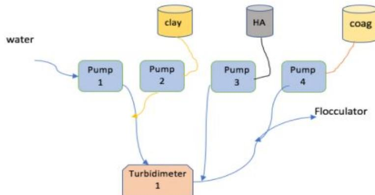
Figure 3: Schematic of experimental apparatus. The second turbidimeter is not shown.
