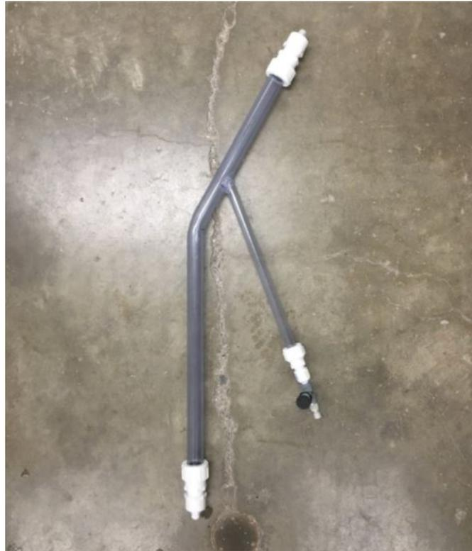
Figure 2: Standardized sedimentation tank
