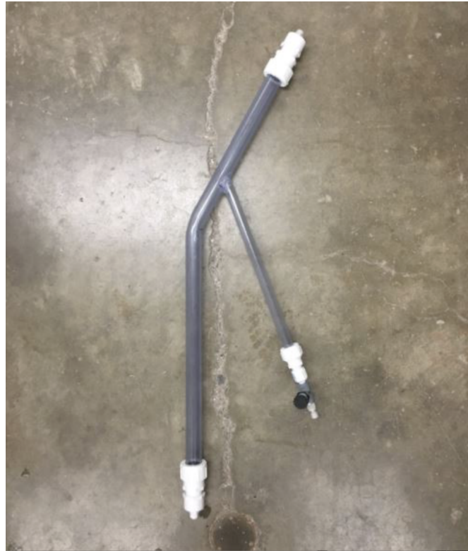
Figure 2: Standardized sedimentation tank
