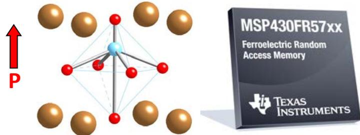
A ferroelectric distortion in the perovskite oxide  $\text{PbTiO}_3$ , one of the materials used in FeRAM devices. The arrow shows the direction of the electrical polarization.
