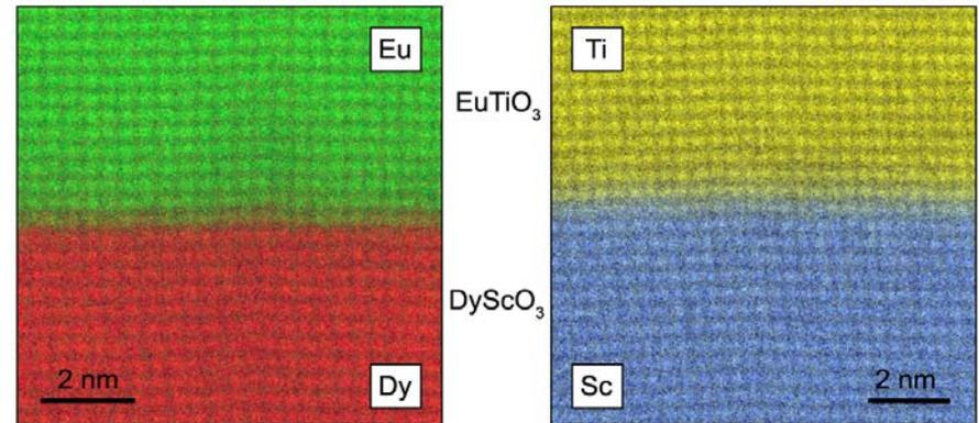
22 nm thick  $\text{EuTiO}_3$  + 1.1% Strain
