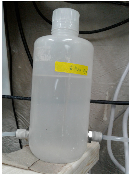
Figure 2: A pressure attenuator is used to even out flow rate during each rotation of the peristaltic water pump.
