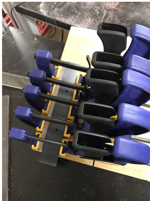
Figure 7: This is how the team used clamps to attach the acrylic to the PVC. This allowed for pressure to be evenly distributed across the flow cell during the drying period.
