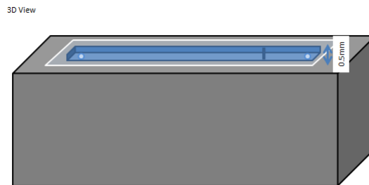
Figure 4: This is the 3D view of the design of the flow cell that the team planned to run experiments with. Flocculated water flows in through microtubing in the first hole, passes through the constriction, shown by a dark line, and exits out the second hole. A glass slide covered the flow cell channel to allow for a clear view of the surface.
