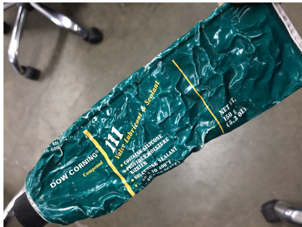
Figure 9: The alternate sealant was used to attempt to create a watertight seal.
