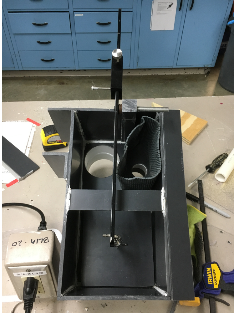
Figure 3: The actual entrance tank shipped to Honduras using the dimensions provided in the AutoCAD file, and fabricated by Juan Guzman.
