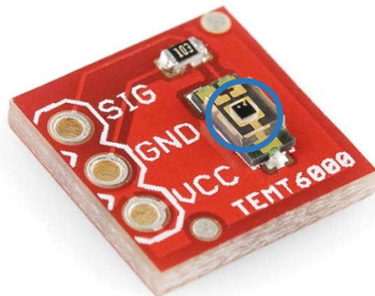
Figure 2: The TEMPT6000 breakout board contains three pins: SIG, GND, and VCC. SIG is the output voltage from the divider circuit. GND is the ground voltage in the circuit of 0 V. VCC is the collector voltage and should not exceed 6 V. Enclosed in the blue circle is the phototransistor, which detects light (Bartlett, 2016).
