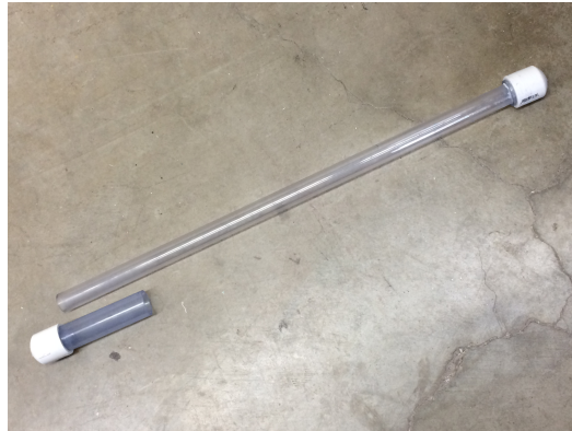
Figure 10: The experimental apparatus modeled after the High Rate Sedimentation recirculator.
