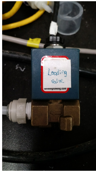
Figure 8: The solenoid valve, which opens and closes to allow gas venting. When the valve is opened, gas is allowed to vent, and the water in the gas sensor drains from the top chamber into the bottom chamber.
