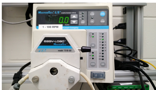
Figure 7: The air pump used to deliver air into the gas sensor.
