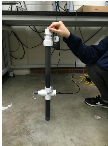
Figure 11: In this figure the photosensor has already been implemented in the testing tube (which already contains the granules inside), and it is fixed with a clamp.
