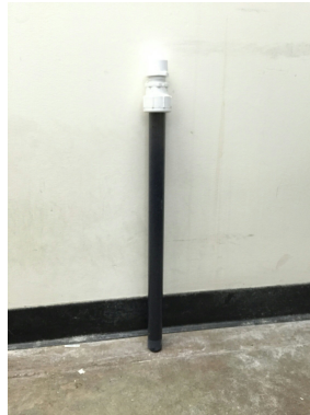
Figure 10: The experimental tube was built to model the tubes in the AFB reactors. Granule samples were taken from the AFB reactors and placed in the experimental tube in varying concentrations to calibrate the photosensor. By measuring the amount of light that passed through the tube, the team designed a calibration curve relating the output in Volts with the concentration of the granules.
