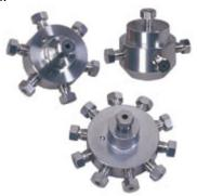
2. They also provide injector/selectors (manifolds) that dial between input lines that all lead into the circle. Just what you may be looking for! <a href="http://www.vici.com/vval/sd.php">http://www.vici.com/vval/sd.php</a> The one showed below, just closes the lines to that are not being used.
