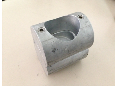
Figure 1: 1.5" Curved Mold currently in use in Honduras. There is only one copy of this mold and therefore it is necessary to document its fabrication details.
